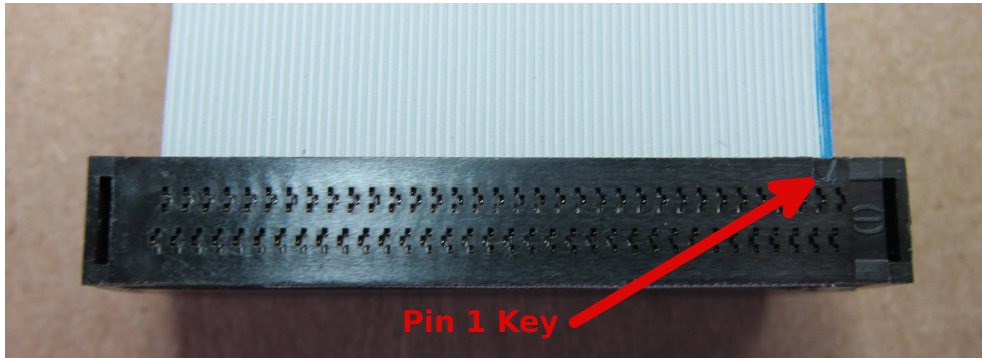
Figure 17: GPIO cable and connector (PCB side).
