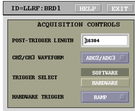
Figure 9: Waveform acquisition configuration panel.
