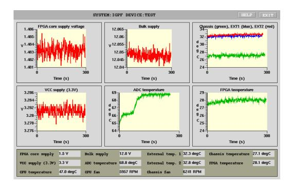
Figure 12: Environmental monitoring panel
