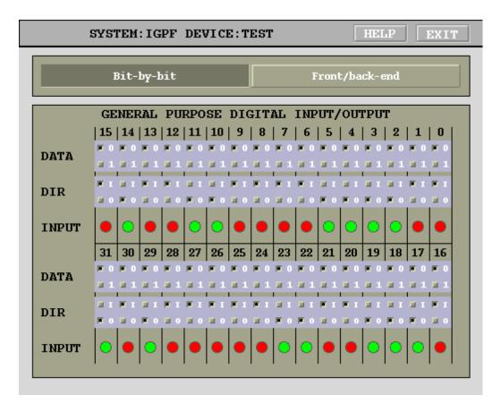
Figure 15: General-purpose I/O panel: bit-by-bit driver
