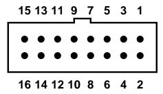
Figure 18: Pin numbering for 16-pin header-type front-panel connectors
