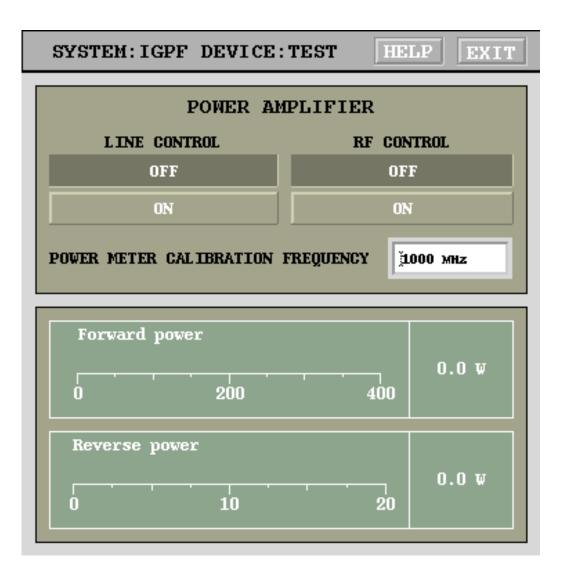
Figure 17: Power amplifier control and monitoring panel
