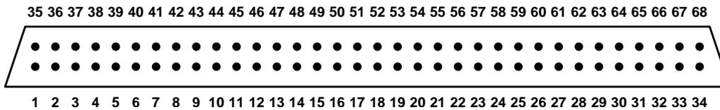
Figure 19: Pin numbering for general-purpose digital I/O connector
