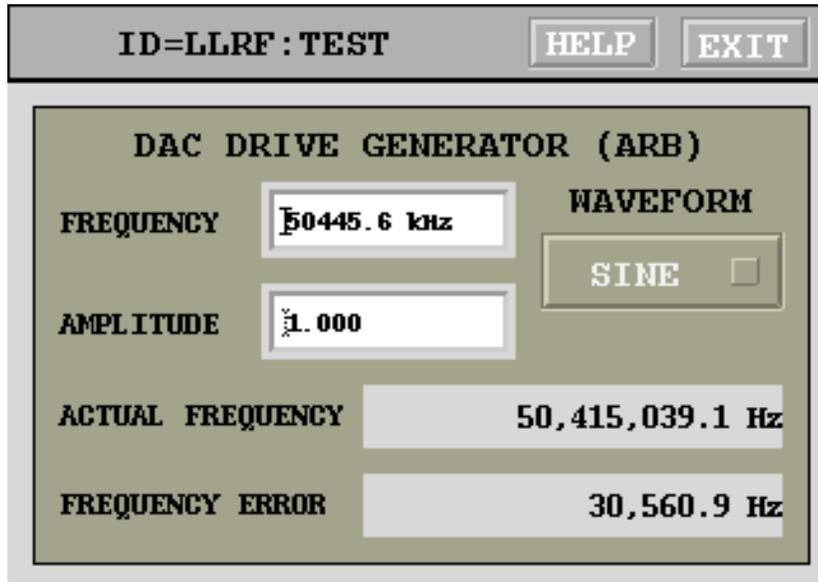
Figure 9: Arbitrary waveform generator panel.
