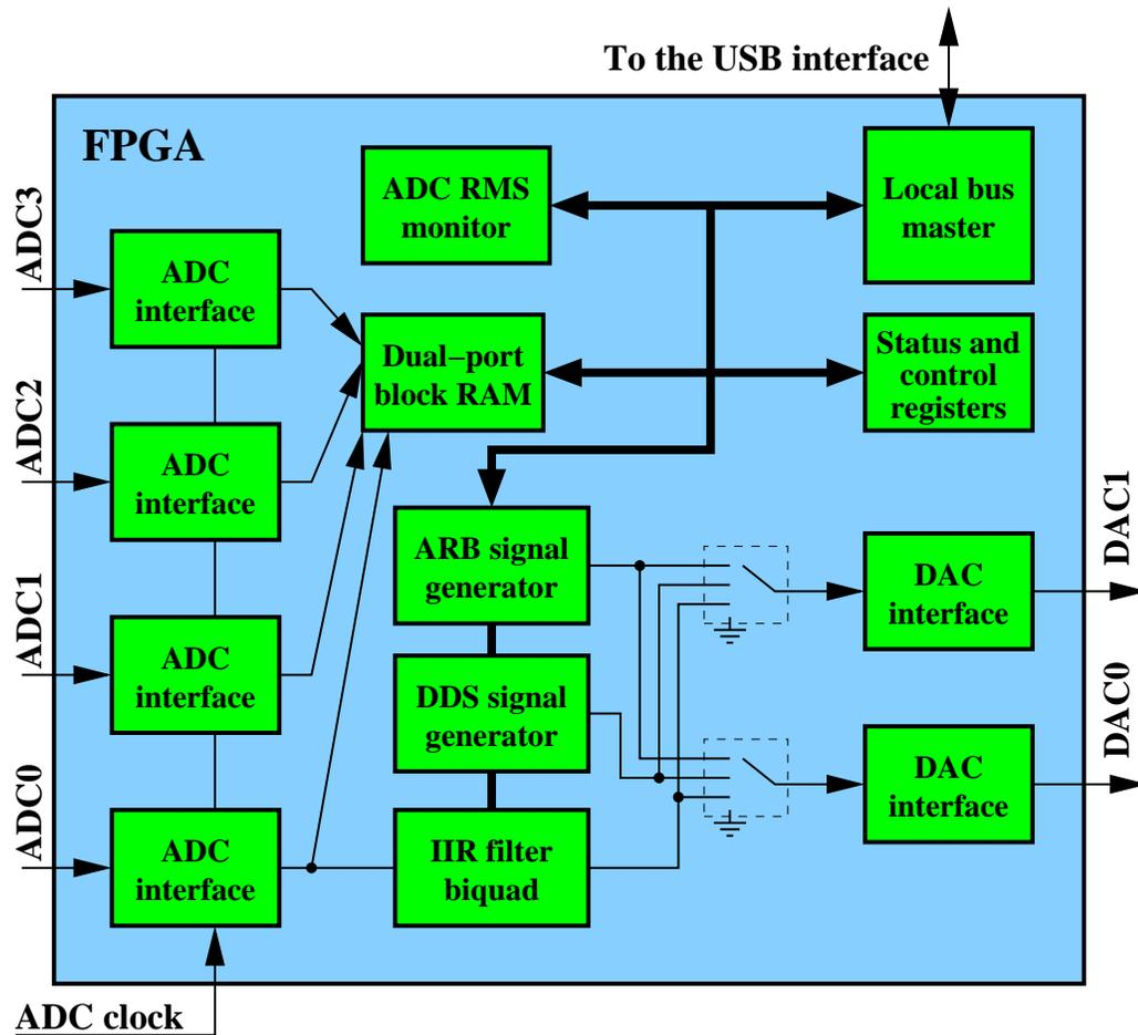
Figure 3: FPGA block diagram.
