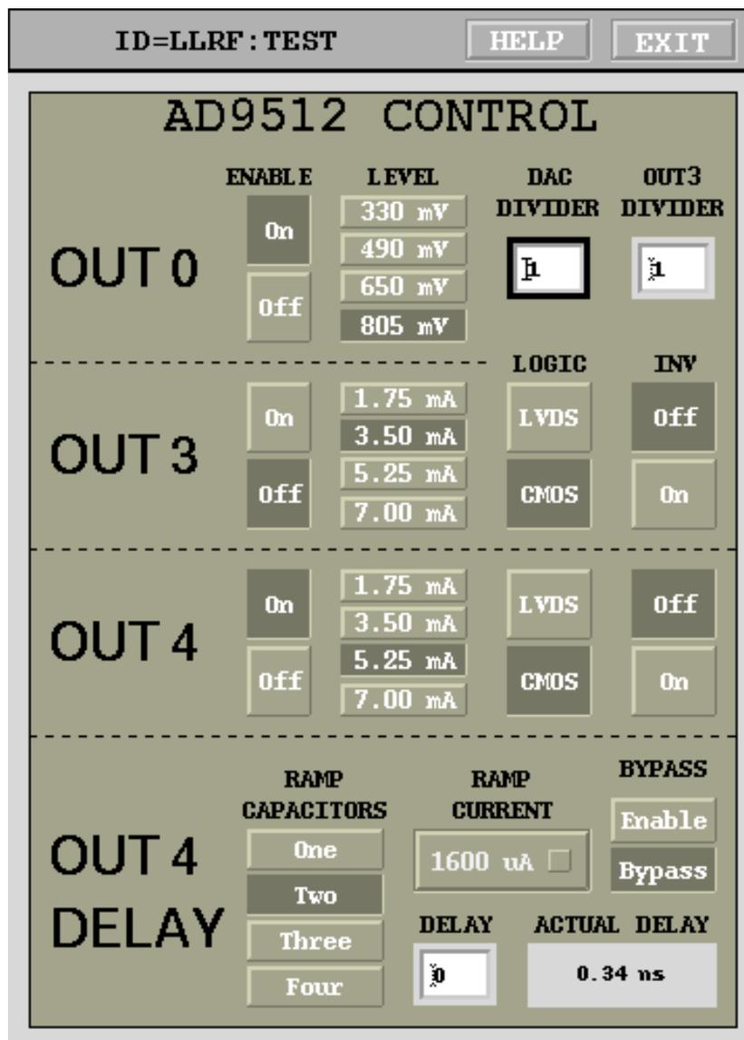
Figure 11: Clock distribution chip controls.
