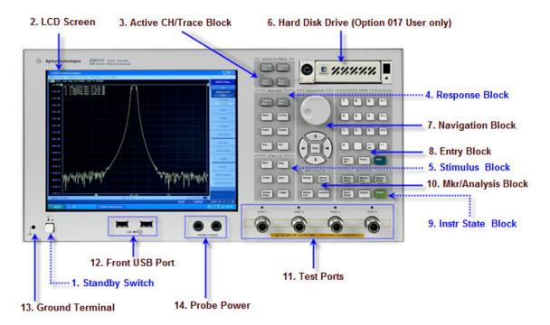
As you can see, there are a lot of buttons, a dial, a screen, some connector ports etc. If you've never worked one of these before it can be a bit overwhelming. So, let's break it into parts:
